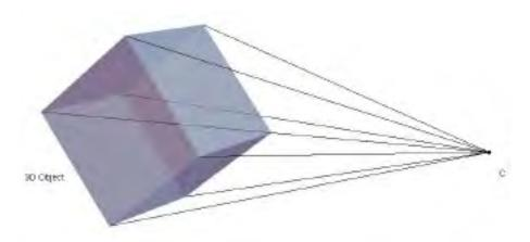
Fig. 3.1. All the rays of the 3D object converge to the camera center,  $\vec{C}$ .
