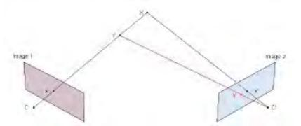
Fig.3.4. If we are using only image 1, depth information is lost because every point on the line  $\overrightarrow{CX}$  (such as  $\overrightarrow{Y}$ ) projects to the same point on the image 1. However, on image 2, different points on the line  $\overrightarrow{CX}$  projects to different points.
