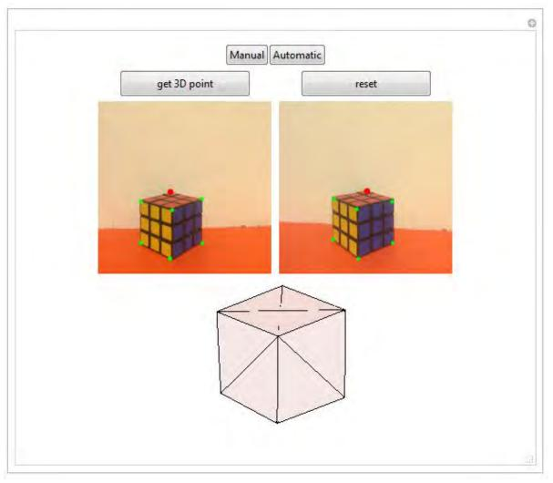
Fig. 5.2. This is the reconstruction with a manual selection of the matching points.
