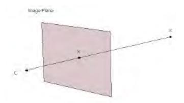
Fig. 3.2. The pinhole camera model.
