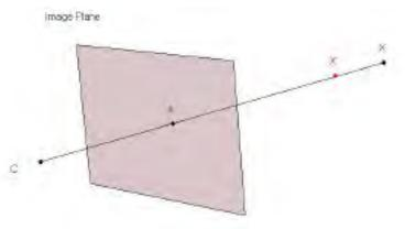
Fig.3.3. Two different points in 3D space  $(\vec{X} \text{ and } \vec{X'})$  will have the same point on the image  $(\vec{O}_i)$ . This shows the important result that depth is lost in a 2D image of a 3D object.
