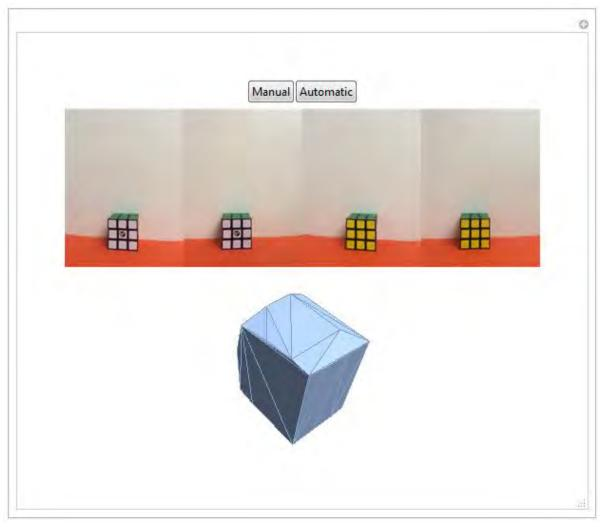
Fig.5.3. This is the reconstruction with an automatic selection of the matching points using the Mathematica function "ImageFeatureTrack".
