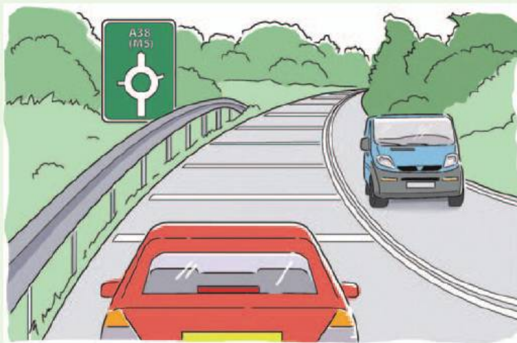
Figure 2.7 Road markings giving a false impression of speed to slow drivers down.
