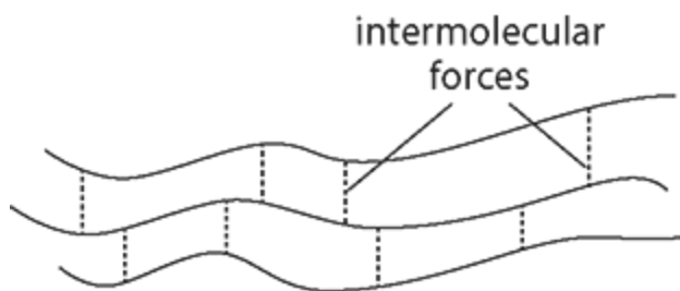
Figure 9.1: Intermolecular forces in a thermoplastic.
