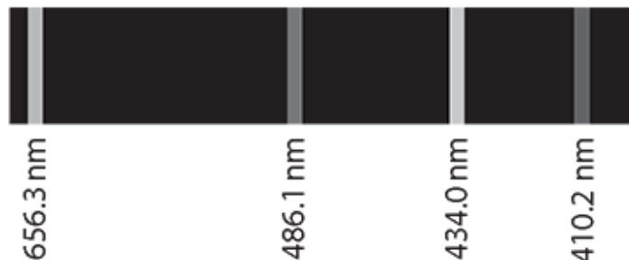
Figure 3.1: Part of the hydrogen emission spectrum.
