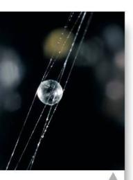
Laser Megajoule fuel pellet. The Laser Megajoule (LMJ) is an experimental nuclear fusion device being built near Bordeaux, France. Its uses laser beams to heat a target to the point where fusion and power generation occurs. It uses the inertial confinement fusion (ICF) method to keep the fuel in place by spider threads.
