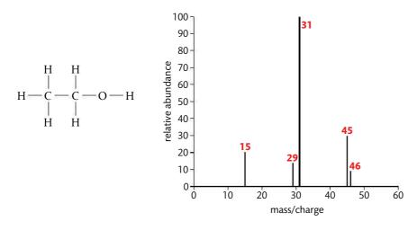
Figure 11.12 The structure of ethanol and its mass spectrum.
