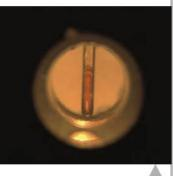
Magnified view through a lens of a melting point determination in a melting point apparatus. The crystals of the sample in the tube are slowly heated electrically until they melt, and the temperature is obtained from a thermometer. Several readings will be averaged and compared with standard literature values to determine the purity of the sample.
