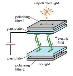
Figure 12.21 Light passes through the LCD despite the orientation of the polarizing filters because the plane of polarization of light rotates with the orientation of the molecules.
