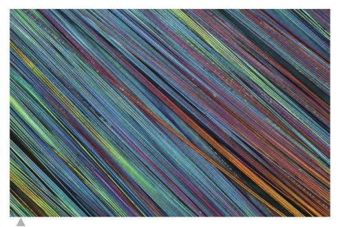
Light micrograph of fibreglass. Fibreglass is a lightweight, extremely strong, and robust material. The plastic matrix may be a thermosetting plastic or thermoplastic.
