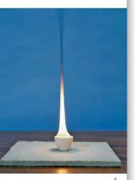
Oct-1-ene, C<sub>8</sub>H<sub>16</sub>, an alkene, burning in a crucible. The flame is smoky due to unburned carbon, an indication of unsaturation.
