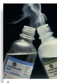
Reaction between vapours of HCI and  $NH_3$  forming the white smoke of ammonium chloride  $NH_4CI$ .
