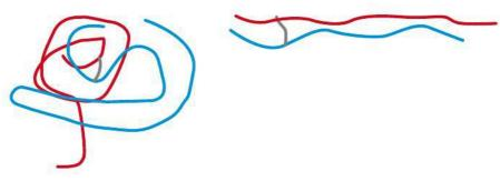
The elastic properties of rubber can be linked to the presence of double bonds in the rubber structure ( $-[CH_2-C(CH_3)=CH-CH_2]_n-$ ), which react with sulfur when the polymer is heated in the vulcanization process. The sulfur atoms form -S-S- bridges between neighbouring chains which keeps the molecule knotted together. The molecules are free to unwind under stress but the cross-links restrict the relative movement between the chains.
