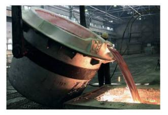
deciding the location of an aluminium plant and they are often sited near hydroelectric power stations. The high energy demand emphasizes the importance of recycling. The energy requirements of recycling aluminium are less than 5% of that needed to extract the metal directly.
