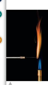
Nichrome wire is used in carrying out flame tests in the laboratory. It is a convenient material because it is resistant to oxidation at high temperatures.
