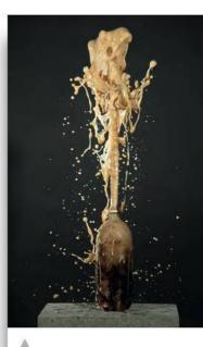
The so-called mentos-soda fountain reaction. Dissolved carbon dioxide in the soda changes quickly into gas in the presence of the candy mint mentos. The sudden pressure change causes the soda to be ejected in a fountain of foam.
