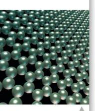
Graphene is composed of hexagonally arranged carbon atoms (spheres) linked by strong covalent bonds. It transports electrons highly efficiently and may one day replace silicon in computer chips and other technology applications.
