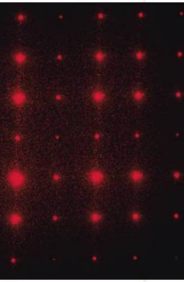
This is a diffraction grating pattern formed by laser light (red), which has passed through an array of crossed gratings. Light is generally considered as a wave.
