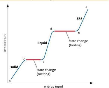
Simple experiments can be done to monitor the temperature change while a substance is heated and changes state. Figure 1.4 shows a typical result. The graph can be interpreted as follows:
