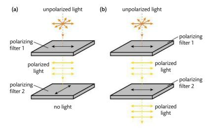
Figure 12.18 (a) When the polarizing filters are crossed so that their planes of polarization are at right angles to one another, no light is transmitted. (b) When the polarizing filters are parallel, all of the light passing through the first filter also passes through the second. The two polarizing filters used together transmit light differently depending on their relative orientations. The second polarizing filter is sometimes called the **analyser**.
