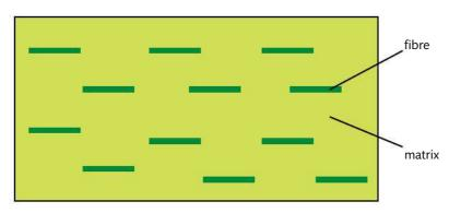
If the composite is designed and fabricated correctly, it combines the strength of the fibre with the toughness of the matrix to achieve a combination of desirable properties not available in any single conventional material. Some composites also offer the advantage of being tailor-made so that properties, such as strength and stiffness, can easily be changed by changing the amount or orientation of the fibre.
