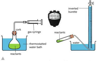
Figure 6.6 Experiments to measure rate of reaction by following change in volume against time.
