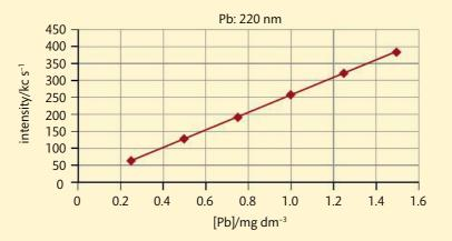
Figure 12.10 A calibration curve for lead.
