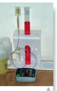
pH testing equipment used to diagnose oesophageal reflux disease. The tubes contain water and buffer solution used to calibrate the sensors and recorder shown at the bottom.
