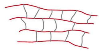
One of the first thermosetting plastics was Bakelite, formed from the co-monomers phenol and methanol (Figure 12.33). Bakelite has a hard rigid structure which does not melt once it has been heated and set. Modern resins are made in a similar way to Bakelite but melamine is used instead of phenol (see Exercise 27).
