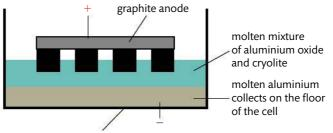
tank lined with graphite cathode
