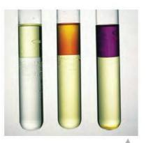
Solutions of chlorine (left), bromine (middle) and iodine (right) in water (lower part) and cyclohexane (upper part). Chlorine dissolves in water, but the halogens are generally more soluble in non-polar solvents like cyclohexane.
