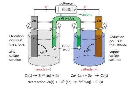
Zinc-copper voltaic cell showing a copper half-cell and a zinc half-cell connected by a salt bridge that appears white. Electrons flow from the zinc electrode to the copper electrode through the electrical wires, while ions flow through the salt bridge to complete the circuit. The voltmeter is showing 1.10 V, the potential difference of this cell.
