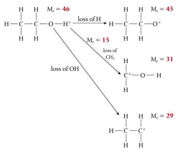
Figure 11.13 Possible fragmentation pattern produced when ethanol is bombarded with high energy electrons.
