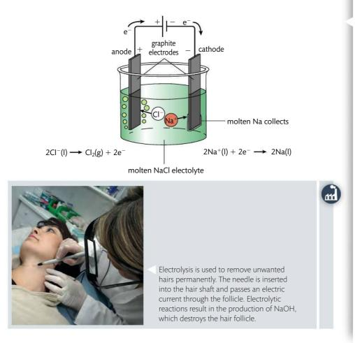
**Figure 9.12** Electrolysis of molten sodium chloride. Chloride ions are oxidized at the anode and sodium ions are reduced at the cathode. The overall equation is  $2NaCl(I) \rightarrow 2Na(I) + Cl_2(g)$ .
