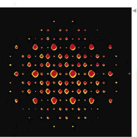
This is an electron diffraction pattern of a binary alloy of 90% titanium and 10% nickel. The pattern can be explained by considering an electron as a wave.
