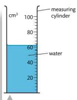
**Figure 11.1** The volume reading should be taken from the bottom of the meniscus. You could report the volume as 62 cm<sup>3</sup> but this is not an exact value.
