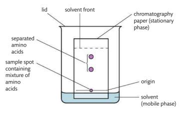
Figure 13.25 Apparatus used to separate amino acids by paper chromatography.
