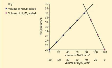
Figure 5.10 Temperature changes produced when different volumes of sodium hydroxide and sulfuric acid are mixed.
