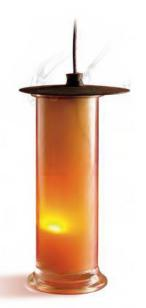
A combustion spoon holding sodium, Na, is lowered into a gas jar containing chlorine, Cl2. The vigorous reaction produces white crystals of sodium chloride, NaCl. 2Na(s) + Cl<sub>2</sub>(g) → 2NaCl(s)
