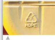
The recycling symbol on the bottom of a bleach bottle indicates that the plastic is high-density poly(ethene). Different plastics can be identified by different numbers. This assists in sorting plastics before they are recycled.
