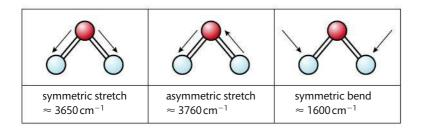
For a symmetrical linear molecule such as carbon dioxide, there are four modes of vibration (Figure 11.18). However, the symmetric stretch is IR inactive as it produces no change in dipole moment. The dipoles of both C=O bonds are equal and opposite throughout the vibration.
