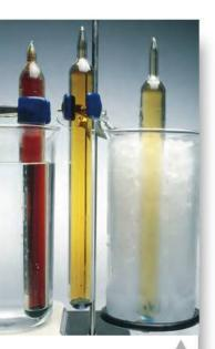
Experiment to show the effect of temperature on the reaction that converts NO<sub>2</sub> (brown) to  $N_2O_4$  (colourless). As the temperature is increased, more  $NO_2$  is produced and the gas becomes darker, as seen in the tube on the left.
