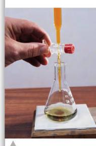
Redox titration experiment. The burette tap controls the flow of the orange potassium dichromate(VI) solution into the conical flask containing iron(II) ions. The equivalence point occurs when the exact volumes of the two solutions have reacted completely.
