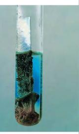
A strip of zinc metal half submerged in a solution of CuSO<sub>4</sub>. Solid copper that appears brown is deposited and the blue colour fades as the copper ions are reduced by the zinc. Zinc is shown to be the stronger reducing agent.
