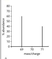
**Figure 2.6** Mass spectrum for gallium. The number of lines indicates the number of isotopes (two in this case), the value on the *x*-axis indicates their mass number (69 and 71) and the *y*-axis shows the percentage abundance.
