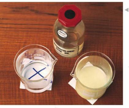
Recording the increase in opaqueness during a reaction. Sodium thiosulfate (left) is a clear liquid, which reacts with hydrochloric acid (upper centre) to form an opaque solution (right). A cross (left) drawn onto paper is placed under the reaction beaker to allow the end point to be confirmed. The experiment is timed from when the reactants are mixed until the cross disappears from sight.
