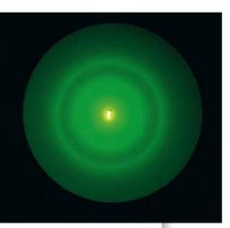
Demonstration of waveparticle duality. An electron gun has been fired at a thin sheet of graphite. The electrons passed through the graphite and hit a luminescent screen, producing the pattern of rings associated with diffraction. Diffraction occurs when a wave passes through an aperture similar in size to its wavelength. Quantum theory shows that electrons have wavelengths inversely proportional to their momentum (momentum is the product of their mass and velocity).
