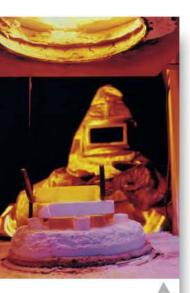
A technologist removing a sample of cermet from a furnace. Cermet is a composite material made from the ceramic boron carbide and the metal aluminium. The cermet is lighter than aluminium but stronger than steel.
