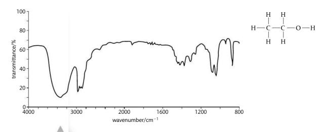
Figure 11.21 The IR spectrum of ethanol. Note that the horizontal axis has a nonlinear scale. This is common for many instruments, so you should always take care when reading off values for the wavenumbers of the absorptions.
