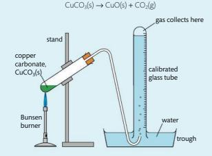
**Figure 1.18** Experiment to calculate the molar mass of carbon dioxide.
