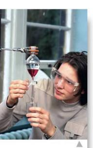
Non-polar liquids like benzene can be separated from aqueous solutions using a separating funnel because they form a separate layer and the lower liquid can be drained. Here, the lower aqueous layer has been coloured purple to make the separation more visible.
