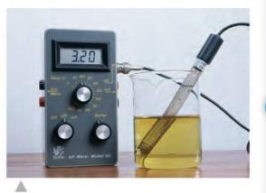
A digital probe showing a pH of 3.20 for the solution in the beaker. The temperature dial is adjusted to the room temperature, allowing the pH meter to compensate for the temperature.
