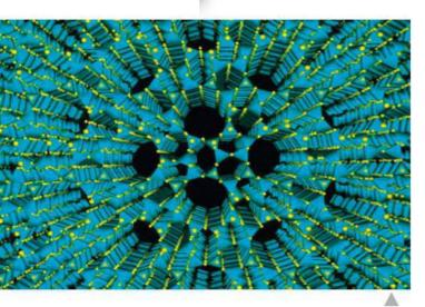
Molecular graphics representation of the structure of the synthetic zeolite catalyst ZSM-5, showing its microchannel architecture. Zeolite minerals containing a silica-alumina crystalline structure are used as catalysts in the cracking process by which crude oil is refined.
