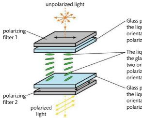
Glass plate is treated to ensure that the liquid crystal molecules are orientated parallel to the first polarizing filter.
