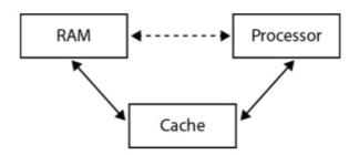
As such, Cache Memory is Smaller and Faster SRAM that temporarily stores the most frequently used data and instructions so that the processor does not need to access the slower primary DRAM. 'Static' means that the memory doesn't need to be constantly refreshed.
