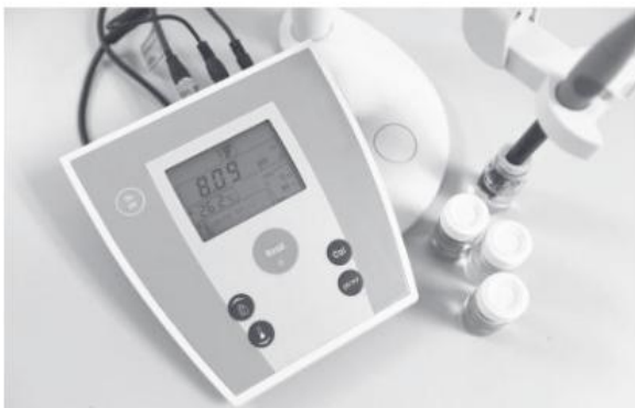
▲ Figure 3.7 Example of a probe with a pH sensor
