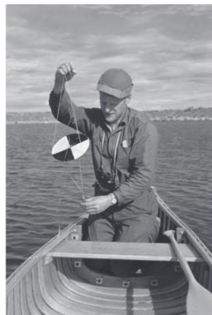
▲ Figure 3.8 A Secchi disc
