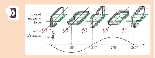
In 1831 **Michael Faraday** discovered that an electric current was generated by rotating a coil of wire in a magnetic field. The electric current produced showed a voltage which varied between positive and negative values as the coil rotated through 360°.
