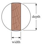
A beam with rectangular cross-section is to be cut from a log of diameter 1 m.
