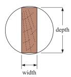
A beam with rectangular cross-section is to be cut from a log of diameter 1 m.
