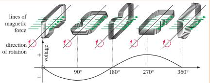
In 1831 **Michael Faraday** discovered that an electric current was generated by rotating a coil of wire in a magnetic field. The electric current produced showed a voltage which varied between positive and negative values as the coil rotated through  $360^{\circ}$ .
