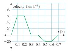
A car travels along a straight road with the velocity-time function illustrated.
