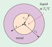
A metal tube has an annulus cross-section with radii  $r_1$  and  $r_2$  as shown.
