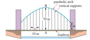
[AB] is the longest vertical support of a bridge which contains a parabolic arch. The vertical supports are 10 m apart. The arch meets the vertical end supports 6 m above the road.
