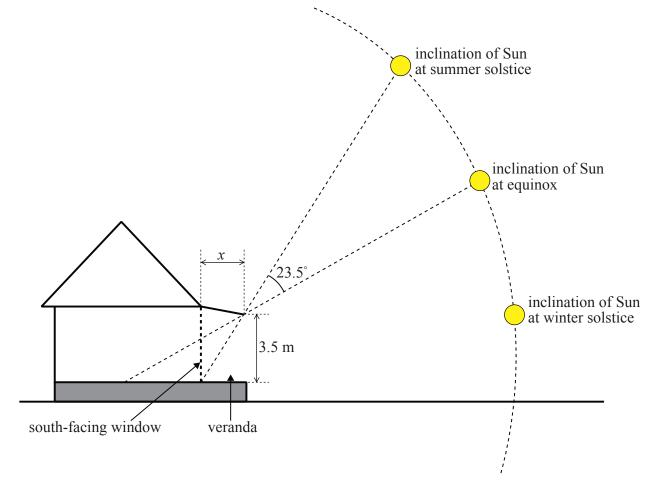
Figure 14: A house located at 45° N where the inclination of the sun at the equinox is 45°
