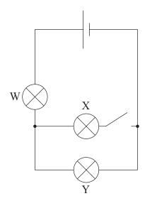
When the switch is closed, all the lamps light. Which of the following correctly describes what happens to the brightness of lamp W and lamp Y when the switch is opened?
