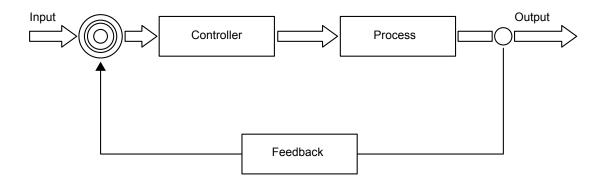
The control system for the electric motor consists of a negative feedback loop.
