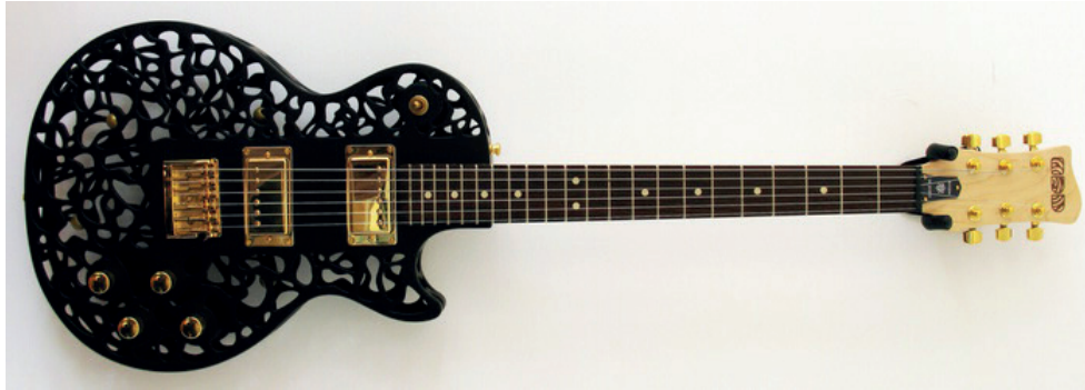
Figure 6: A 3D printed guitar body
