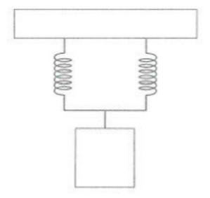
The time period of the oscillation for the two-spring system is  $T_2$ .
