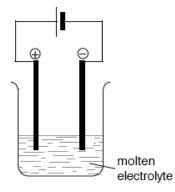
molten electrolyte/MgCl<sub>2</sub>(I), electrodes and battery/DC supply;
