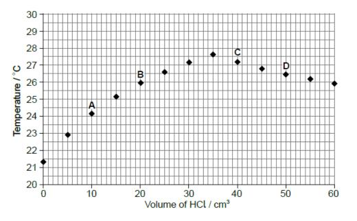
A class was determining the concentration of aqueous sodium hydroxide by titrating it with hydrochloric acid, whilst monitoring the pH of the solution. The sodium hydroxide solution was added into a glass beaker from a measuring cylinder and the hydrochloric acid added using a burette. One group of students accidentally used a temperature probe rather than a pH probe. Their results are given below.
