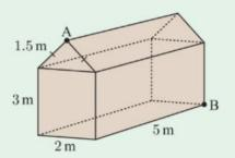
A barn has the dimensions given. Find the shortest distance from A to B.
