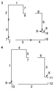
Note: The following is only one possible solution. The numbers show how the 9 skirting boards are used. Joins are indicated by 'x'. Board 1 is 3200 mm long (100 mm waste) Boards 2, 3, 4, 5, 6 are 3300 mm long. Board 7 is cut into 3 pieces (1000 mm, 400 mm, 1800 mm) Board 8 is cut into 4 pieces (600 mm, 1600 mm, 700 mm, 300 mm) Board 9 is cut into 2 pieces (900 mm, 400 mm) If joins at corners are not counted the smallest number of joins possible is 4.
