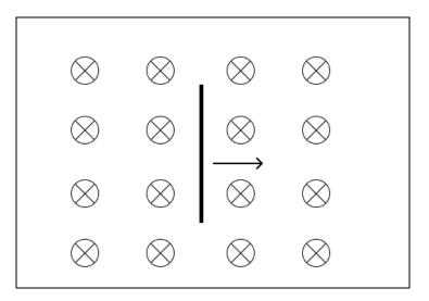
The wire moves at a speed of 4.0 m s<sup>-1</sup>. What are the magnitude of the emf and the direction of current inside the wire?
