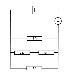
The cell has an internal resistance of 2  $\Omega$  and the ammeter reading is 2 A. What is the emf of the cell?
