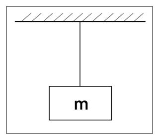
The student hypothesizes that the change in length is given by the following formula:  $\frac{\Delta L}{L} = \frac{F}{EA}$  where L is the original length of the wire, A is the cross-sectional area, F is the force applied to the wire, and E is a constant.
