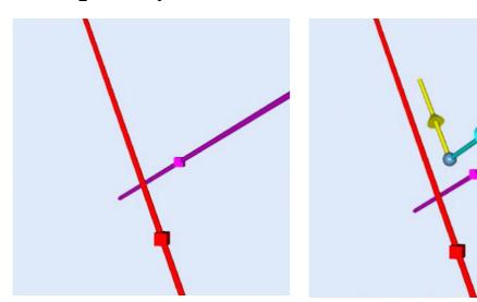
Angle between lines = Angle between direction vectors parallel to the lines
