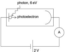
If the work function of the target is 3 eV what is the maximum energy of electrons reaching the anode?
