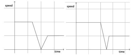
If the scales on each graph are the same how is the impulse and force different?
