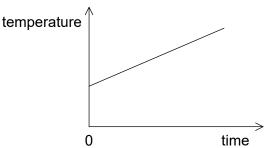
If the power supplied is P and the gradient of the line k, what is the heat capacity of the metal cube?
