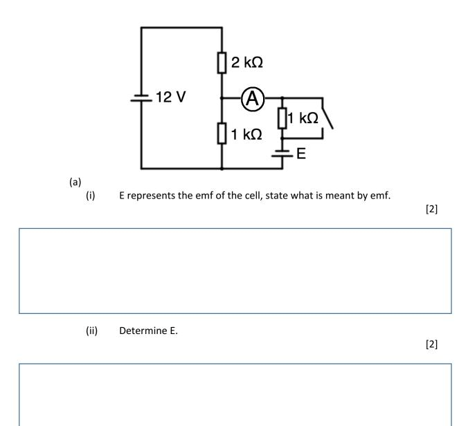
(iii) Deduce the effect, if any, that closing the switch would have on the ammeter reading.
