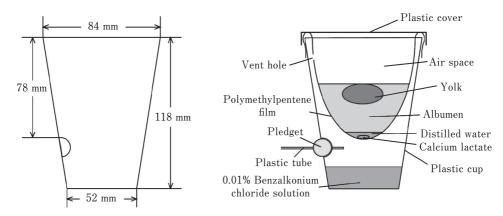
Fig. 3. Schematic drawings of the artificial culture vessel used for chicken embryo culture.
