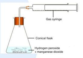
In three separate experiments the volume of oxygen evolved was measured over time when no manganese dioxide was added, when 0.100 g of manganese dioxide was added and when 1.00 g of manganese dioxide was added to the same volume of hydrogen peroxide solution. The temperature was kept constant throughout.
