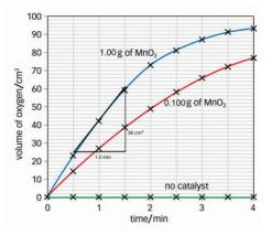
(c) Determine the rate of reaction after one minute when 1.00 g of manganese dioxide had been used as a catalyst. [1]
