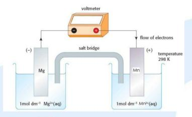
Cell potential = 1.18 V (the difference between – 2.37 V and – 1.19 V)
