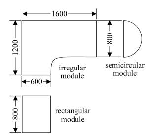
The modules used to create the L-shaped layout shown in the picture.
