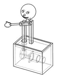
relationship cam - push rod; relationship motor / gearbox - cam; 3D correct; do not penalise if only cam and push rod shown.
