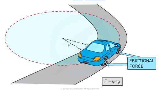
• Therefore, in order for a vehicle to avoid skidding on a curved road of radius  $\it r$ , its speed must satisfy the equation
