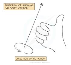
Wrap the right hand around the axis of rotation so that the fingers are pointing in the direction of rotation. The thumb points in the direction of the angular velocity vector
