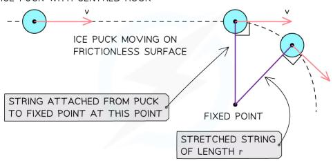
The applied force (tension) from the string causes the puck to move with uniform circular motion
