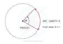
When the angle is equal to one radian, the length of the arc (S) is equal to the radius (r) of the circle
