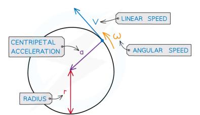
Centripetal acceleration is always directed toward the centre of the circle and is perpendicular to the object's velocity
