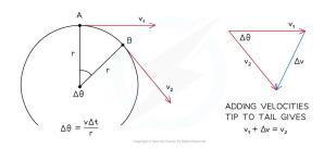
Slide a ruler parallel to  $\Delta v$  towards the circle. Midway between A and B,  $\Delta v$  points towards the centre of the circle. This is the same direction as the centripetal acceleration
