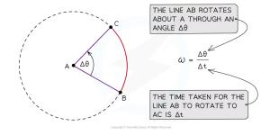
The angular speed is  $\omega$  is the rate at which the line AB rotates
