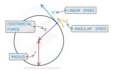
Centripetal force is always perpendicular to the linear velocity (i.e., the direction of travel)
