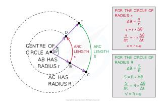
The angle  $\Delta\theta$  is swept out in a time  $\Delta t$ , but the arc lengths s and S are different and so are the linear speeds
